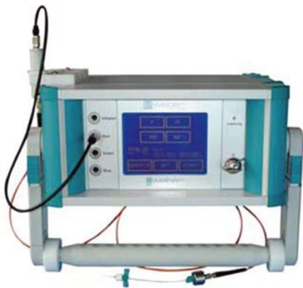
Picture 6: Certified laser blood irradiation system with biocompatible disposable catheters, Source: M. Weber [53]
