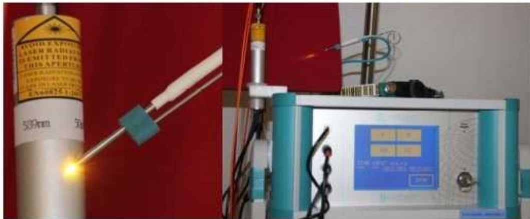
Fig. 2: First yellow laser (589 nm, 50 mW) for future medical applications at the Medical University of Graz.
